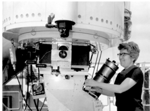
Vera Rubin, with DTM image tube spectrograph attached to the Kitt Peak 84-inch telescope, 1970.
