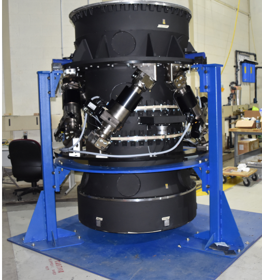
Fig. 10: Based on core capabilities and expertise developed in the DECam project, Fermilab played major roles in construction of the outer ring, barrel, cage, hexapod, and ADC rotator for the DESI project (at left), including testing with a state-of-the-art, large-scale coordinate-measuring machine at SiDet.
